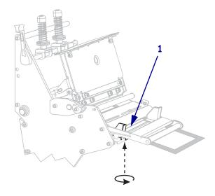
**10.** Push down the printhead assembly (1), and then rotate the printhead-open lever (2) clockwise until it locks into place.
